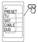
To change the labels, press the SCROLL button repeatedly. Each time the SCROLL button is pressed, the labels change as in Step 4 on page 14. When the desired component is selected, the component name (in this case, TV) and the four-digit component code number previously set to the component is displayed.
